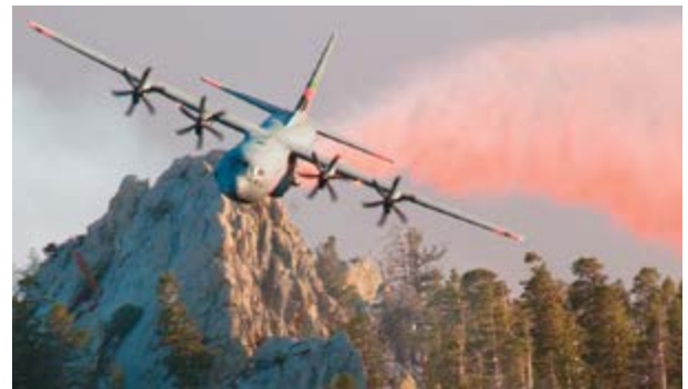
A California Air National Guard C-130J Hercules cargo transport from the 146th Airlift Wing in Port Hueneme, California, drops fire retardant on the Mountain Fire in Palm Springs on July 19, 2013. The aircraft is outfitted with a Modular Airborne Fire Fighting System (MAFFS), a self-contained unit used for aerial firefighting that can be loaded onto a C-130 to allow the aircraft to be used as an air tanker against wildfires.
