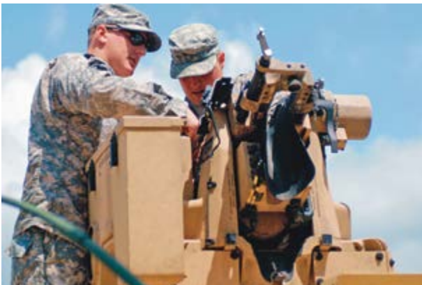
PFC Longo and PFC Esters observe the mechanics of the CROWS II system during their first day approach training at Camp Grayling, Michigan, July 15, 2012. A soldier is in the cab maneuvering the site picture on the system.
